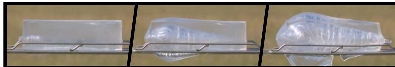
180 grain Premier Scirocco Bonded bullet shot from 300 WIN Mag. showing devastating expansion and energy transfer on gel.
