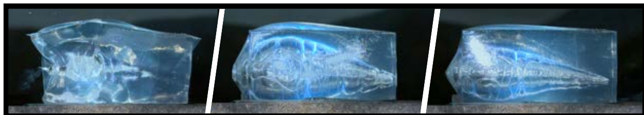
High speed videography time lapse of ballistic gel testing shows extreme energy transfer and wound channel expansion. Premier Long Range 172 grain .308 WIN @ 200 yards shown.
