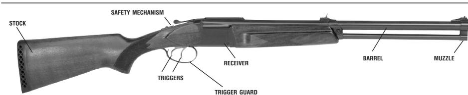
*This picture shows the main parts of a Remington Model SPR94 Over and Under Combination rifle/shotgun. The picture will aid in understanding the instructions in this book.*
