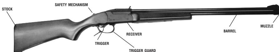
*This picture shows the main parts of a Remington Model SPR94 Over and Under Combination rifle/shotgun. The picture will aid in understanding the instructions in this book.*
