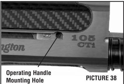
10. Turn the operating handle 1/4 turn clockwise to lock into place.
