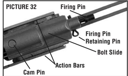
insert the firing pin retaining pin (cotter pin) into hole. See Picture 32.
