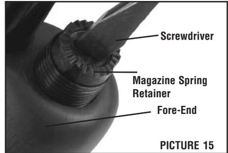
6. Push down on the screwdriver and magazine spring retainer approximately one (1) inch or until you can turn the screw driver.
