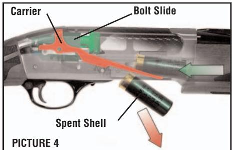
After the shell is ejected, the carrier moves the new shell released from the magazine (Picture 5) and places it in front of the bolt. Completing the cycle, the bolt moves forward chambering the new shell. See Picture 2. Once the last shell has been discharged, the bolt assembly locks in the open position.
