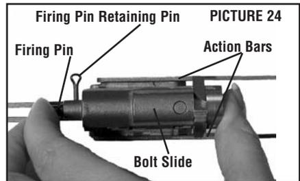
2. Slowly release the firing pin and remove from the bolt assembly.
