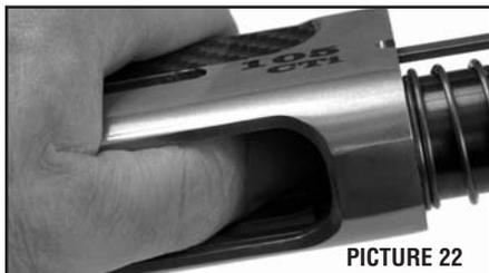
2. Push the bolt to the top of the receiver while sliding the action sleeve assembly and bolt assembly forward from the receiver as a unit. See Picture 22.
