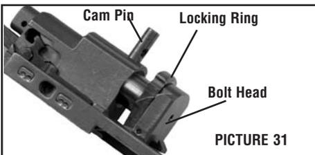
5. Reassemble the firing pin assembly by placing
