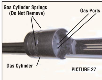
13. Spray Rem™ Action Cleaner in the gas cylinder. Push a wire brush the size of the gas cylinder through the gas cylinder several times and wipe dry. **DO NOT REMOVE THE GAS CYLINDER SEAL OR GAS CYLINDER SPRINGS.** See Picture 27 and 28.
