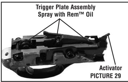
3. Apply a light application of Rem™ Oil to the locations as shown in Picture 29.
