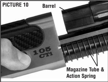
8. Once the barrel bottoms out in the receiver, slowly release the operating handle.
