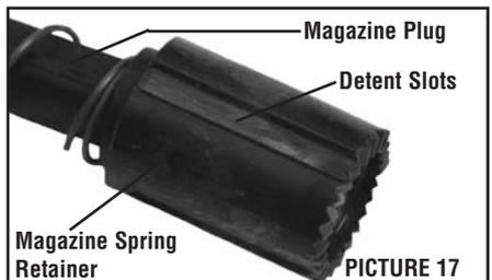
11. Push the magazine spring, plug, and retainer into the magazine tube while aligning the magazine spring retainer detent slots with the detents in the magazine tube. See Picture 17.
