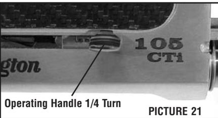
1. With the barrel and trigger plate assembly removed and the bolt closed, turn the operating handle counter clockwise 1/4 turn and remove. See Picture 21.
